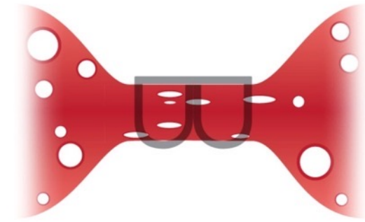
Energy is stored in the staple as compression is maintained
